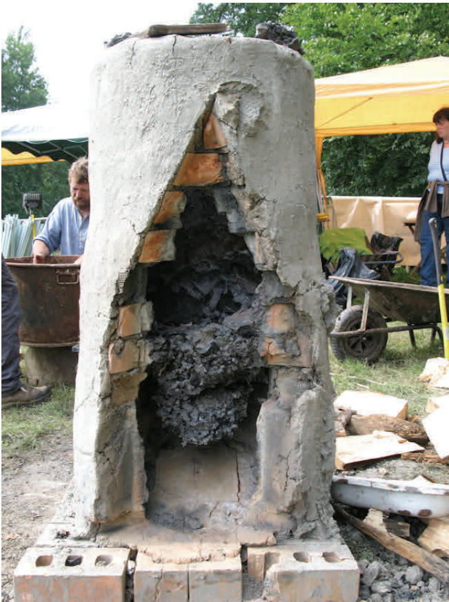
Fig. 1 Furnace sectioned part way through a smelt and emptied of charcoal to show progress of forming a bloom.
