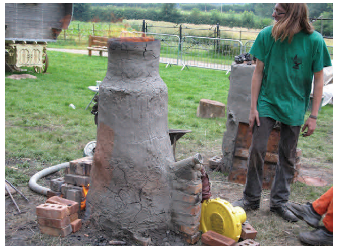
Fig. 3 The German furnace showing rear tuyere and additional air blown at front to encourage slag flow.
